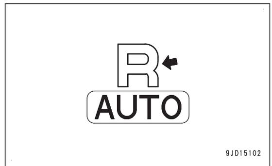
While the back grade mode indicator is displayed on the control box screen, you can control the dozing in forward travel by setting the joystick (steering, directional and gear shift lever) to FORWARD position (F). You can perform the back grade work by setting the lever to REVERSE position (R).
