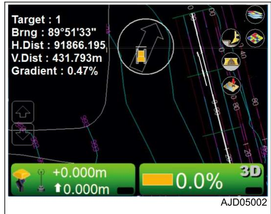
When the point to navigate to and the machine are displayed on the same screen, the arrow goes out.
