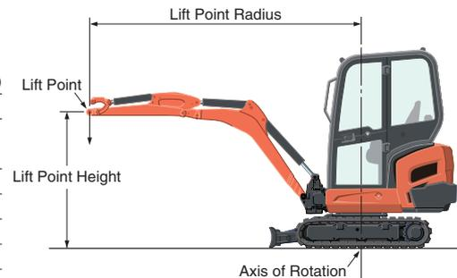
\*The lifting capacities are based on ISO 10567 and do not exceed 75% of the static tilt load of the machine or 87% of the hydraulic lifting capacities of the machine.
