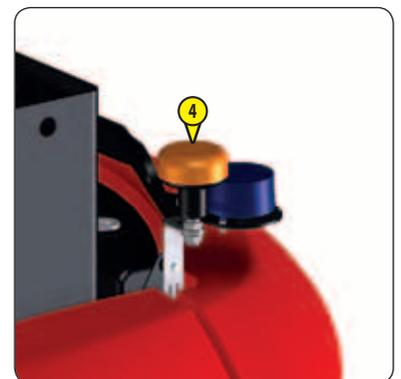
**DEACTIVATE OR ACTIVATE THE ENGINE AUTOMATIC STOP SYSTEM "STOP AND GO"**
