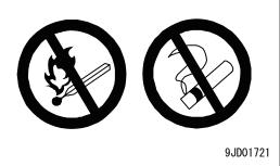
KDPF is a device to purify the soot in the exhaust gas. Exhaust gas temperature may increase during the aftertreatment devices regeneration. Do not bring any combustible material close to the outlet of the exhaust pipe.
