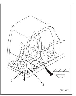
9. Fit the floor mat and secure it by inserting projections (2) into the holes.
