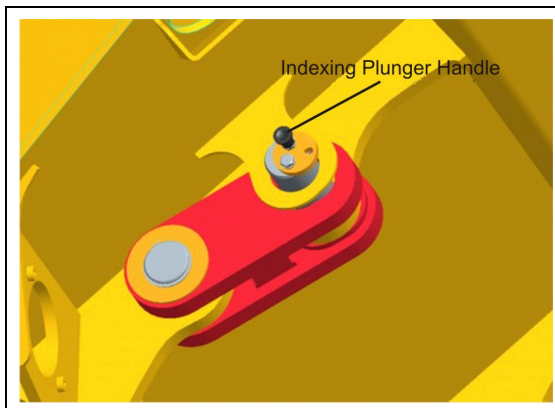
Figure 1: Over Centre Bin Lock Feature (Male Clevis)
