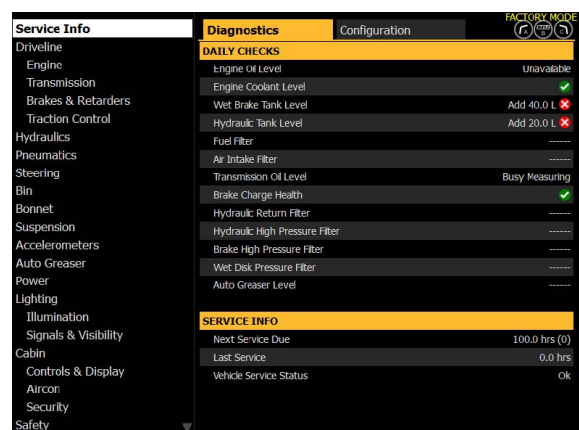
Daily Checks Menu illustrating the quantity of oil required in the WDB and Hydraulic tank.
